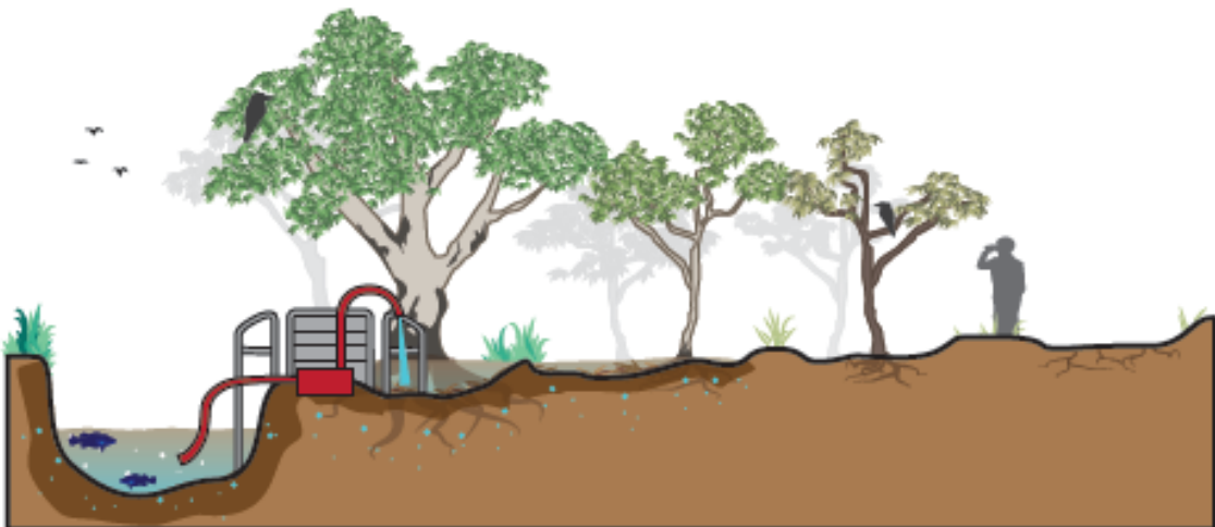
Scenario 3: If the floodplain is too dry, we can use a temporary pump to get environmental water onto the floodplain and close the regulators to hold the water there for as long as needed, before returning the water to the river.
