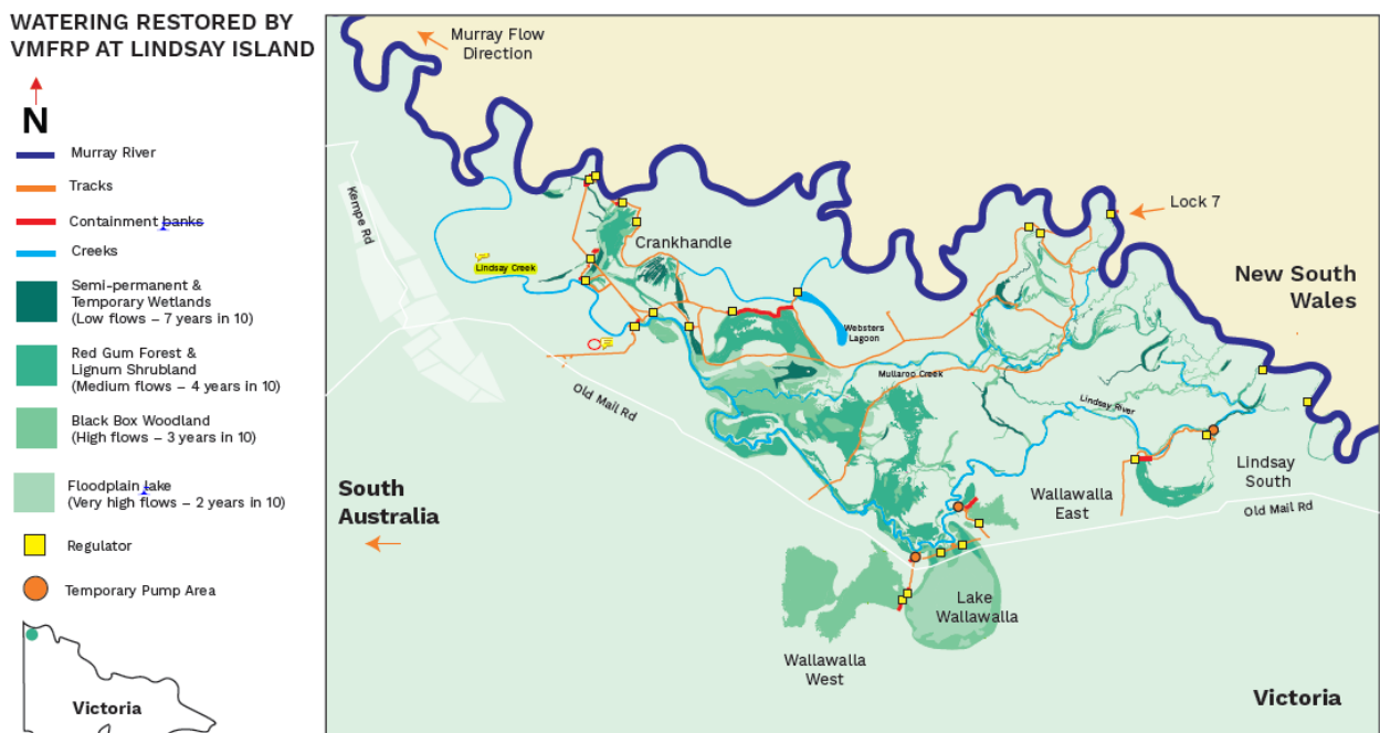
Figure 2: Extent of vegetation that can be reached with VMFRP works (based on conceptual design from October 2021)
