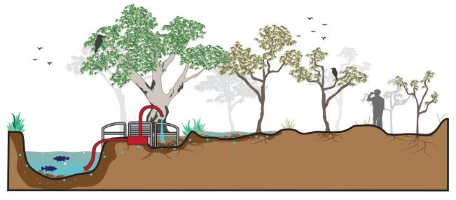
Scenario 3: If the floodplain is too dry, we can use a temporary pump to get environmental water onto the floodplain and close the regulators to hold the water there for as long as needed, before returning the water to the river.
